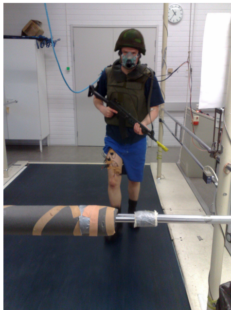
FIGURE 19. The military simulating combined strength and endurance loading contained treadmill run/walk with the military gear.
